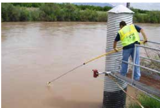
Figure 13: EBID staff collect a sample for E. coli analysis at the Leasburg gage on the Rio Grande.
